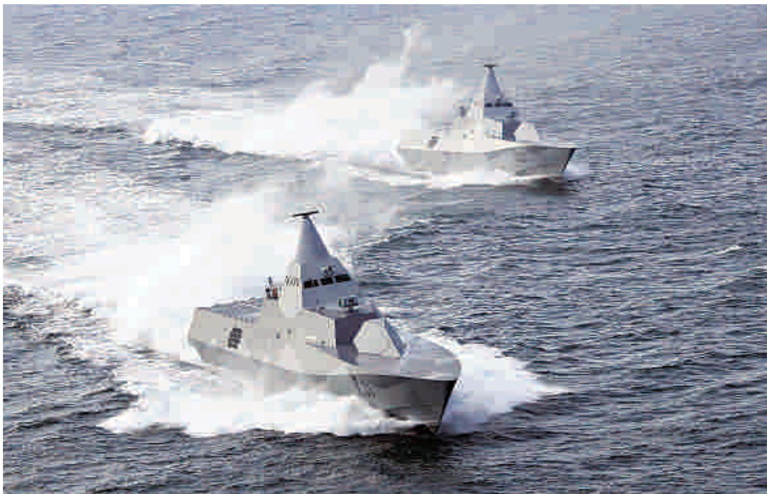
**Sweden's 620-ton Visby-class corvettes employ stealth technology and are equipped for anti-surface and anti-submarine warfare as well as mine countermeasures missions.**
